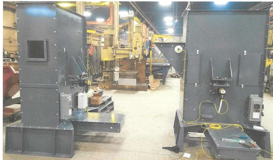
Boot on Pedestal with Cleanout Slide Gate. Requires a Head Take-up (not shown)
