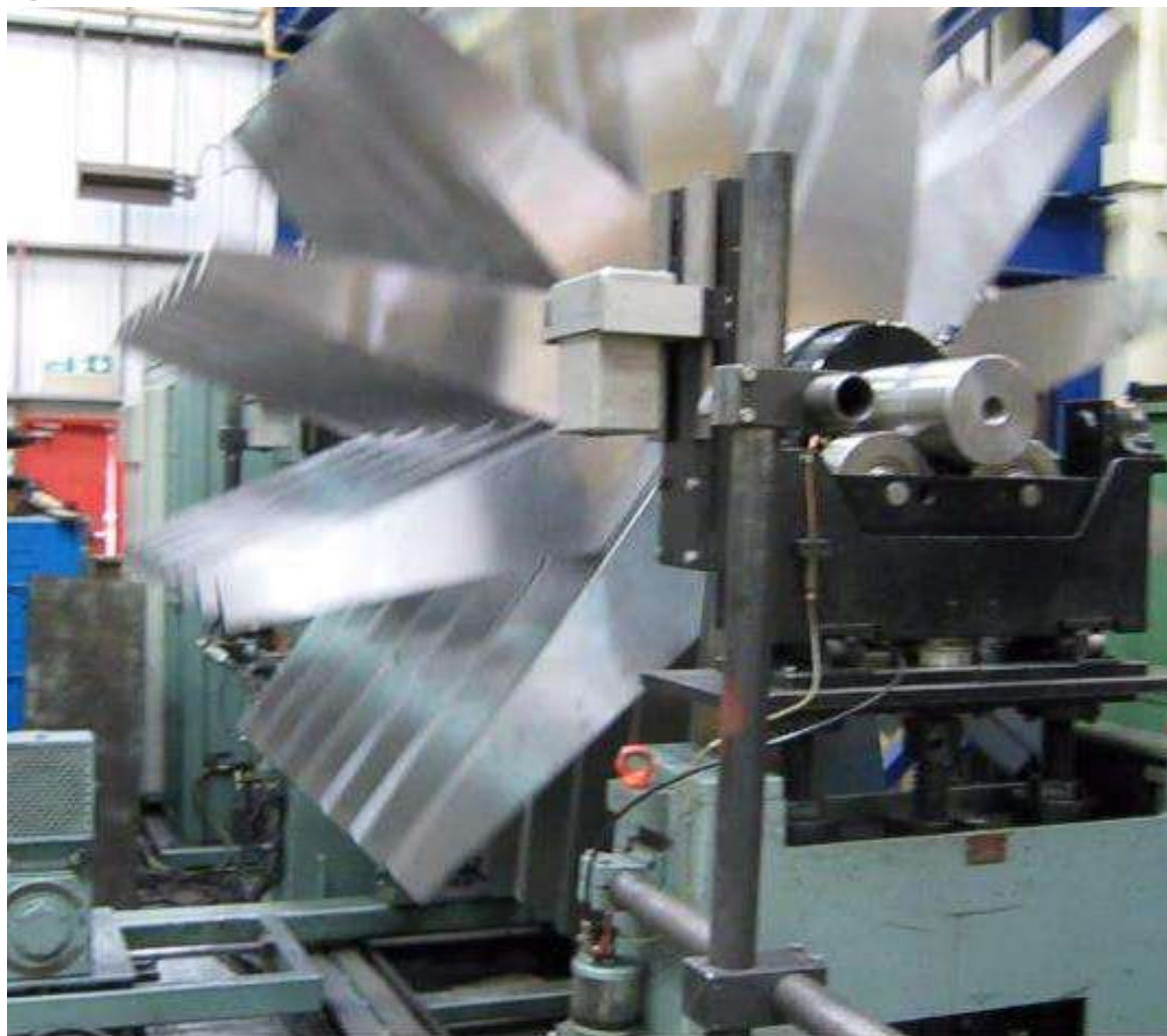
Disintegrator Rotor undergoing Dynamic Balancing
