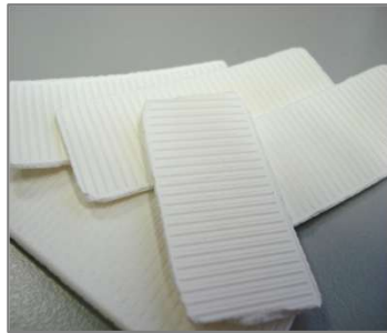
Compacted sheet (roll compaction)
