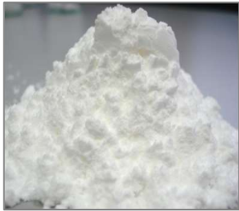
Initial powder (poor flowing)
