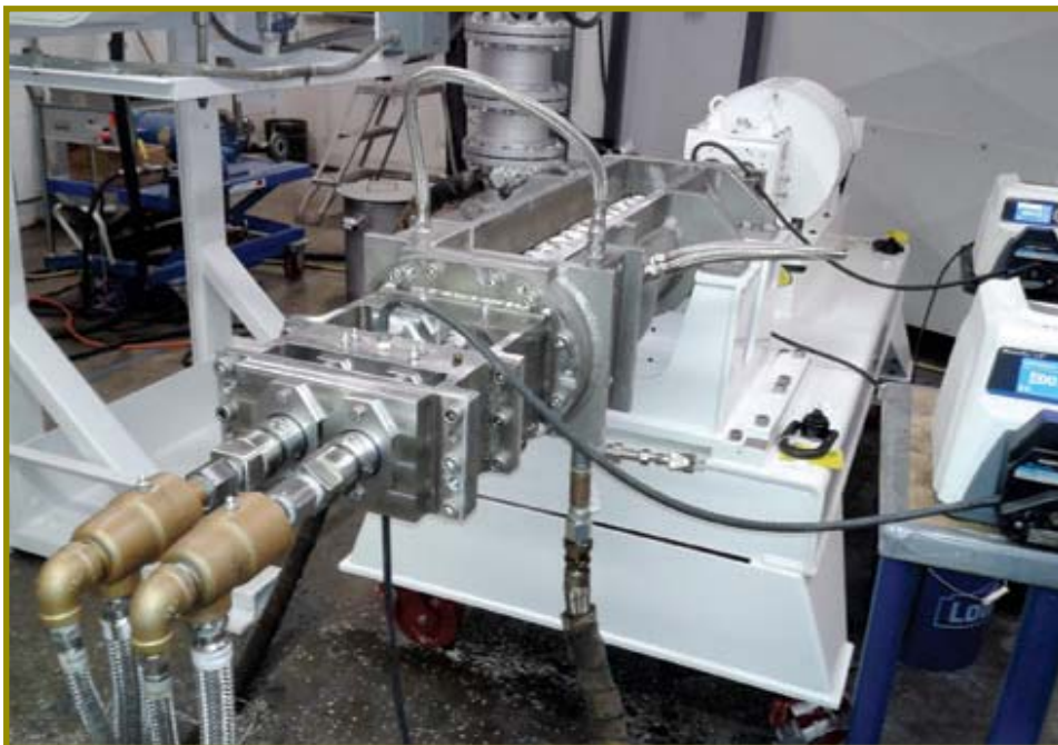
The SCP, by Readco Kurimoto, thickens liquids or changes liquids into powders. PHOTO/SUBMITTED
